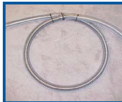
Figure 3: Cable Coil Placed Inside Slit Tube
